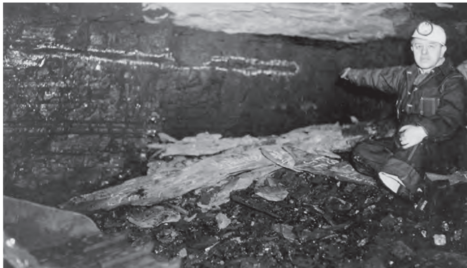
Outline of rib hole after shooting on left rib at face of 8 west, 22 south. This shot suspected of causing explosion.
