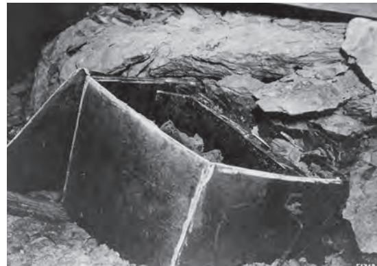
Black (pellet) powder storage box, found following explosion with front side blown off.
