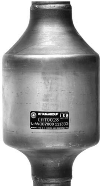
A new catalytic converter with an identifying stamp designed to prevent theft.
