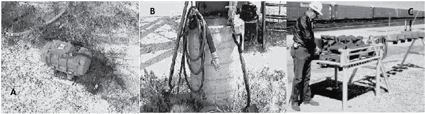
Figure 7. (a) heavy railcar shaker “stored” on the ground, (b) poorly organized tools and hoses, (c) improved rail yard organization and storage: storage table for coupler knuckles allows lifting at waist height rather than from ground.
