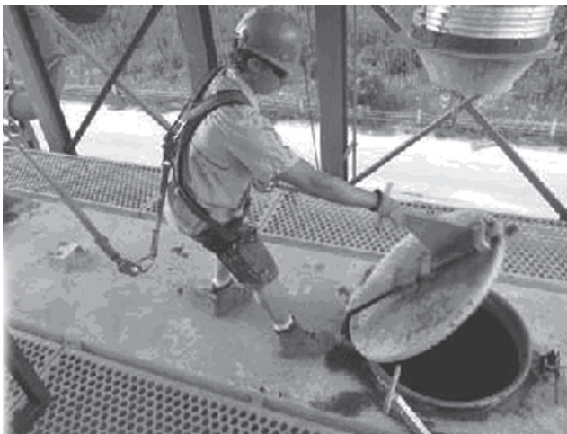
Figure 4. Opening covered hopper car hatches (a) manually and (b) using rail hatch opener.
