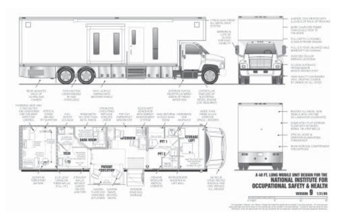
Figure 2. Schematic drawing of the van.
