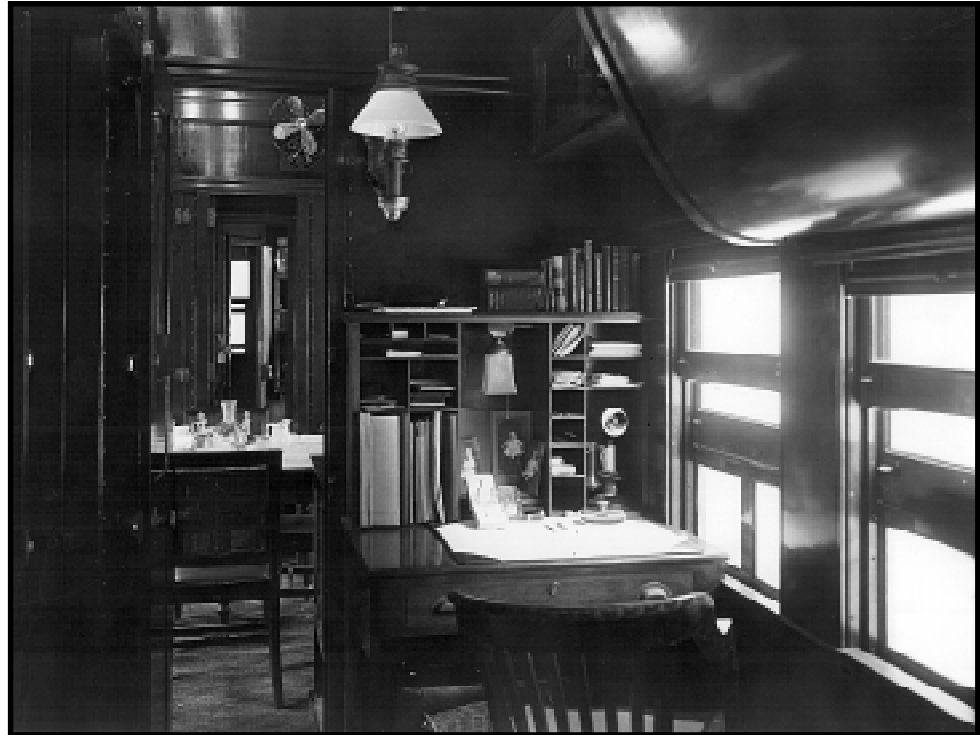
Office compartment on Car No. 11. There is an electric light over the desk and a gas light on the bulkhead.
