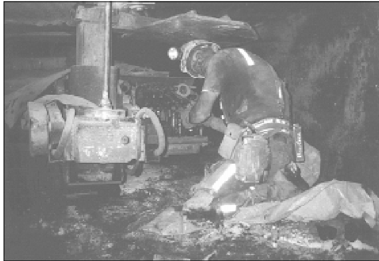
Roof bolting in a low-seam mine often requires operators, such as this one, to maintain awkward postures.
