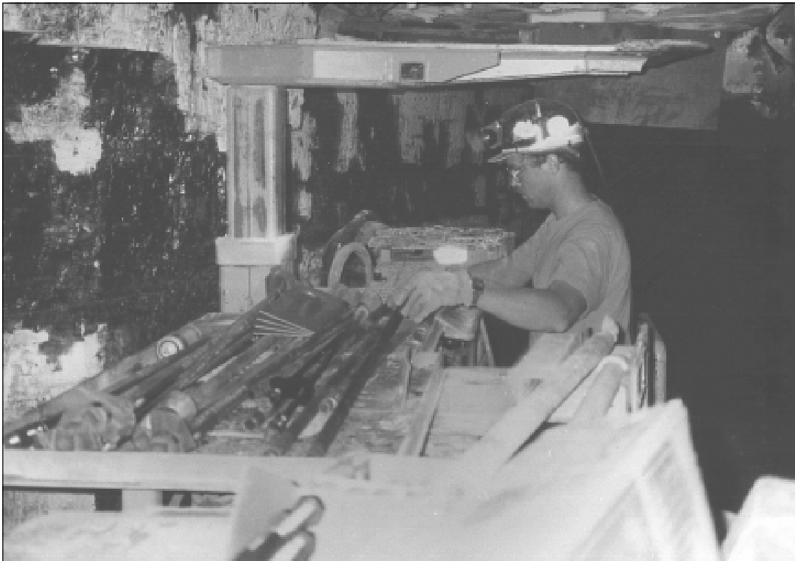
Figure 2.— Bolter operator retrieving supplies from a tool tray mounted on a bolting machine
