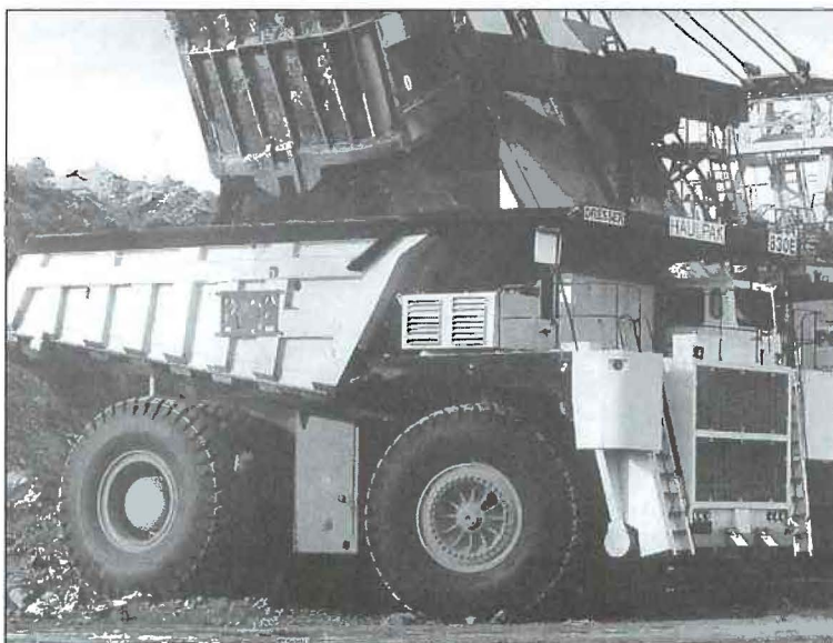
◀ Left: An electric shovel dumps a load of overburden into the bed of a 240-ton haul truck at Jacobs Ranch Mine. Use of these trucks, the largest available to the industry, has increased productivity and efficiency.
