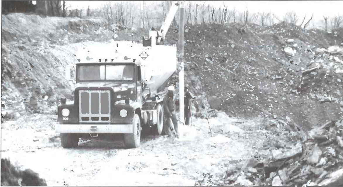
Independent contractor blaster filling drill hole with explosive at surface mine
