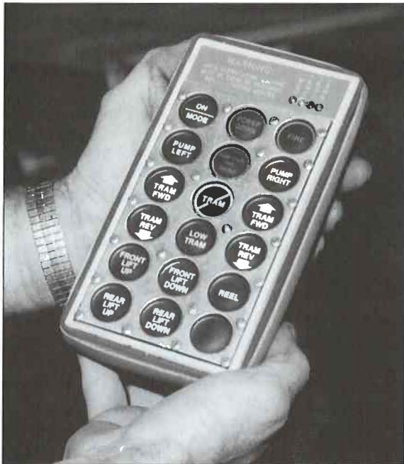
A hand-held remote control enables a roof bolter to move the machine from a distance of up to 200-300 feet in line of sight.
