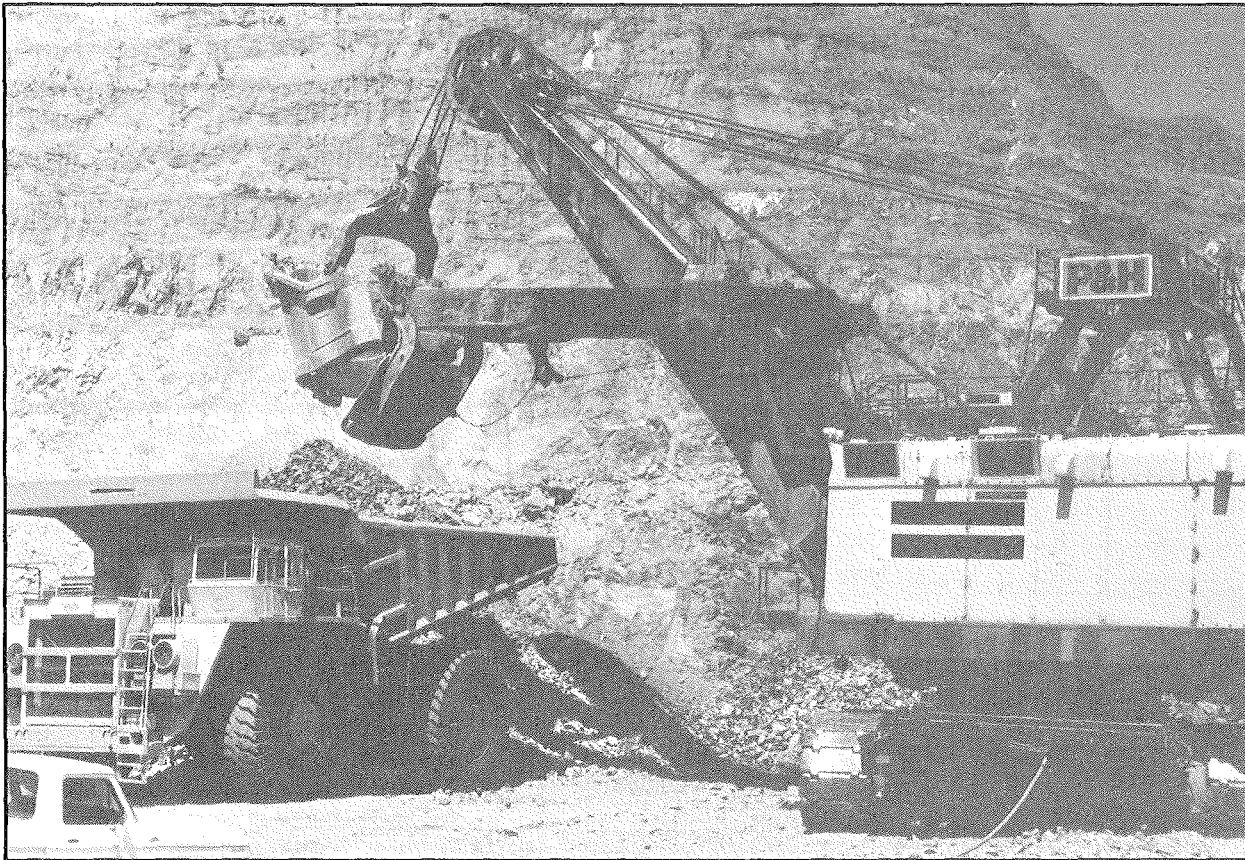
Injuries to haul truck drivers can occur while the truck is being loaded if the operator is not adequately protected against loading shocks. Loading shocks can occur due to the bucket striking the truck body or from large boulders being dropped into the bed.
