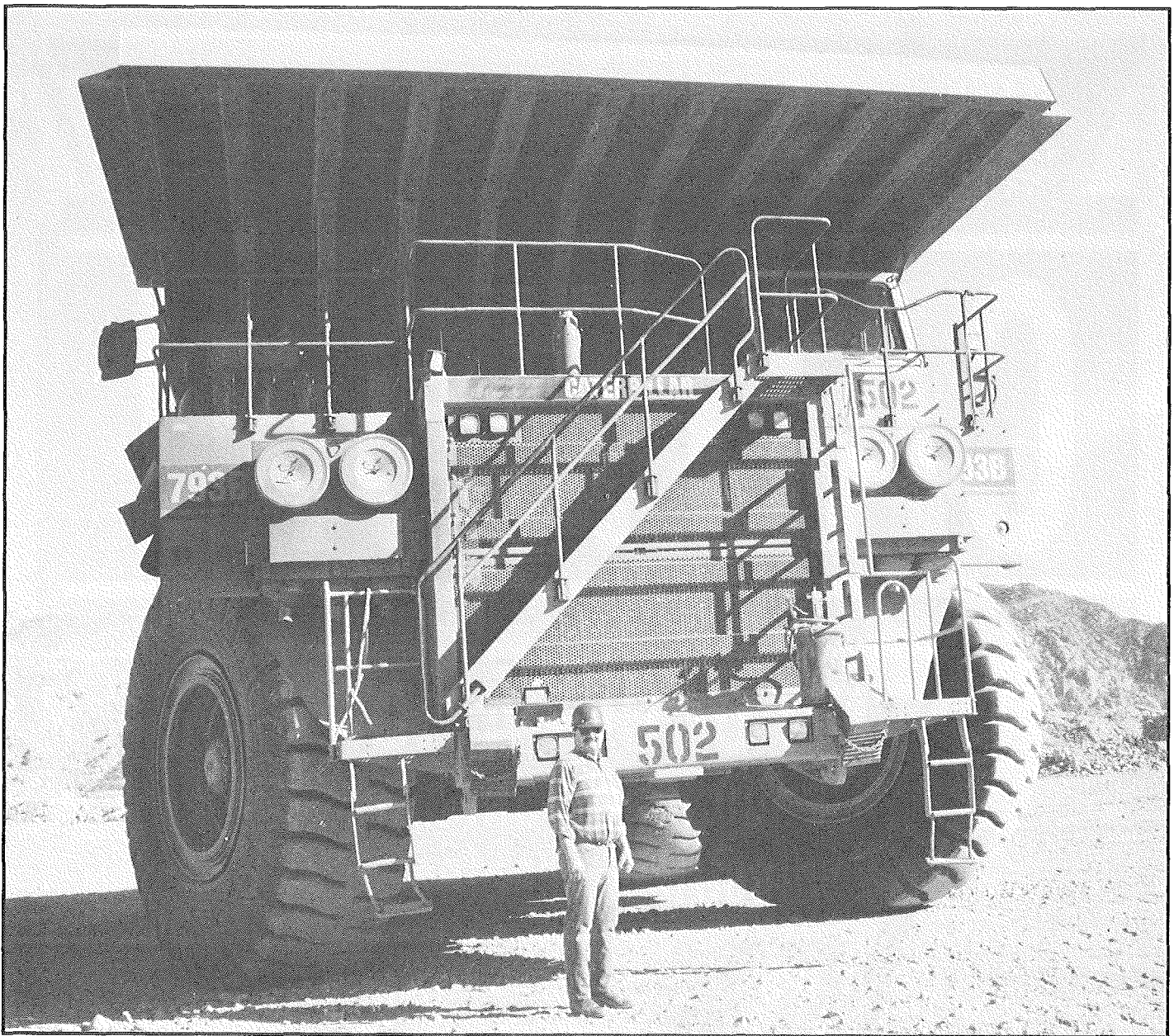
One person—one truck—240 tons per trip. Armando Abril with his new haulage truck, far removed from one man, one shovel
