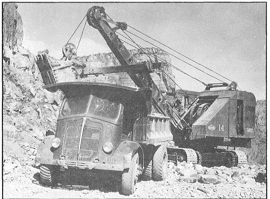
In the early days of the Morenci open pit, trucks such as this one, with a capacity of only 5 cubic yards, about 7 tons, were employed in the mine—especially in confined areas. This photo was taken in April 1939.
