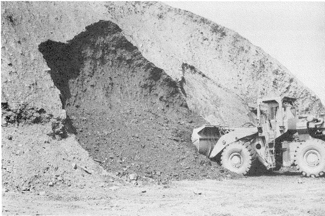
Figure 3.—Loading out from toe can create dangerous condition.
