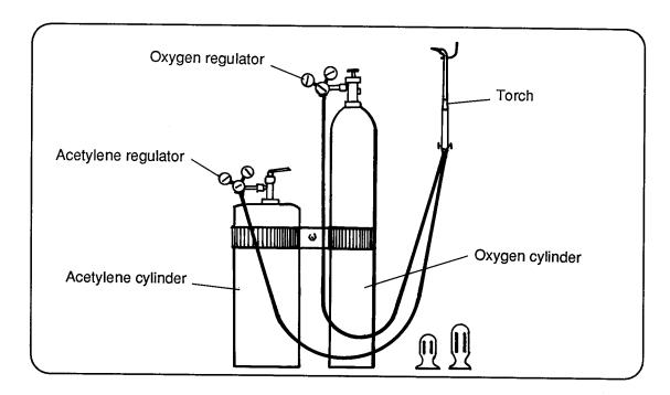
Hoses used for oxyacetylene welding have to conform to the Compressed Gas Association's standards for rubber welding hoses. These hoses are usually siamese. The red hose is used for fuel gas and the green hose for oxygen.
