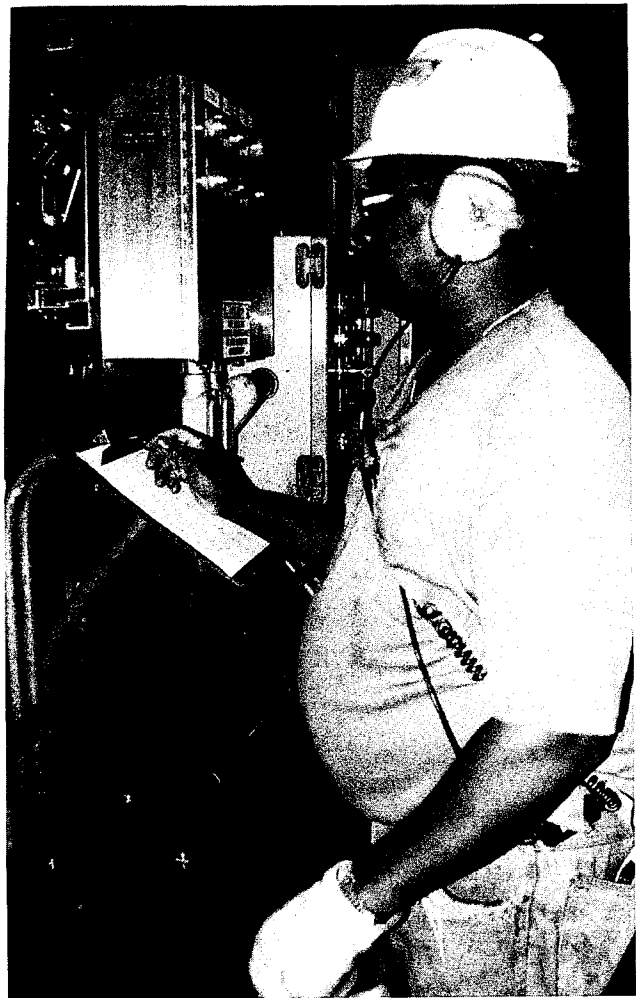
Andy Avery, a stationary equipment operator at the plant, has hearing protection that doubles as a receiver for communicating with refuse truck drivers
