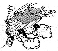
Avoid applying brake continuously on a long downgrade unless system is so designed. Use engine for additional brake force — or, if so equipped, the auxiliary retarder.
