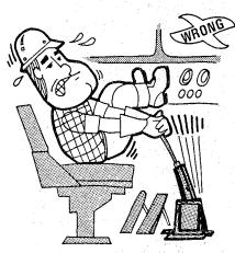
Use the parking brake ONLY for parking. While an emergency may possibly justify using this brake to help slow truck —
