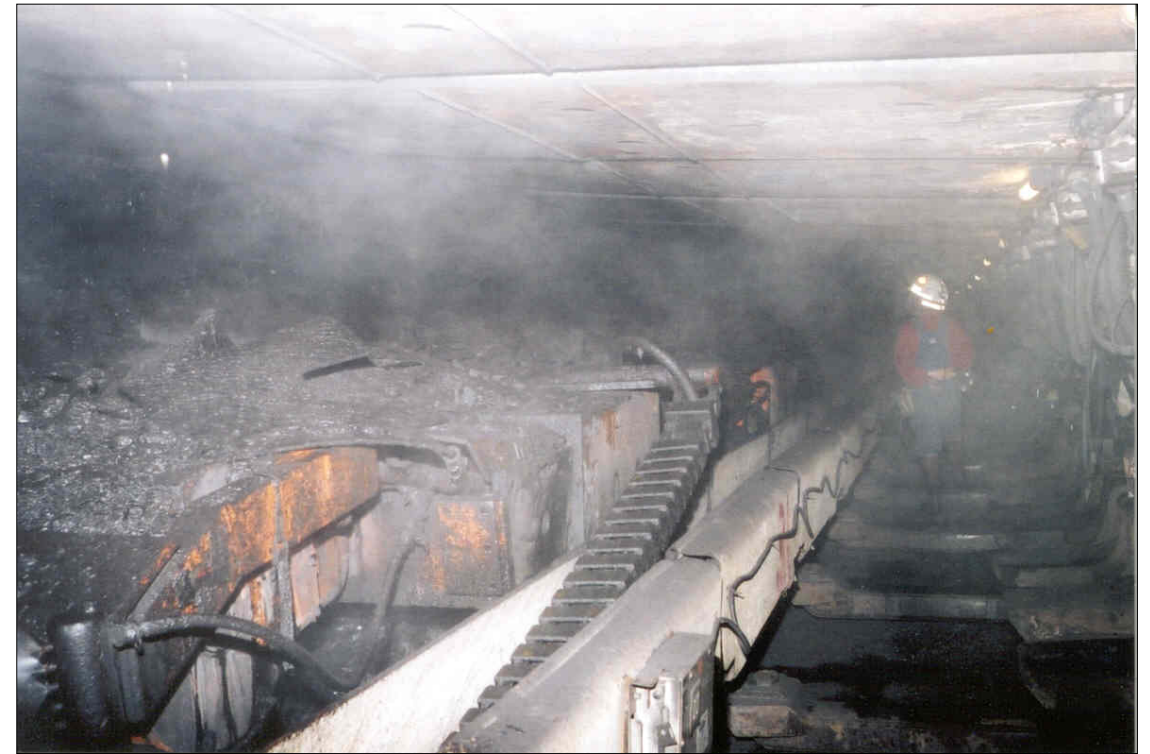
Ineffective directional sprays allow dust to roll into walkway
