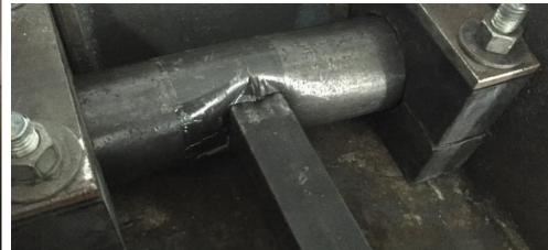
Modified Hopkinson-Bar device for high strain-rate experiments
