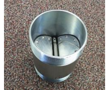
Steel Check Valve
