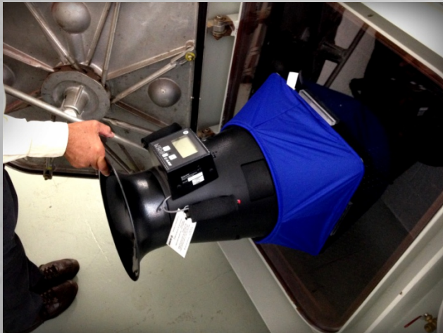
Measuring air flow from air curtain
