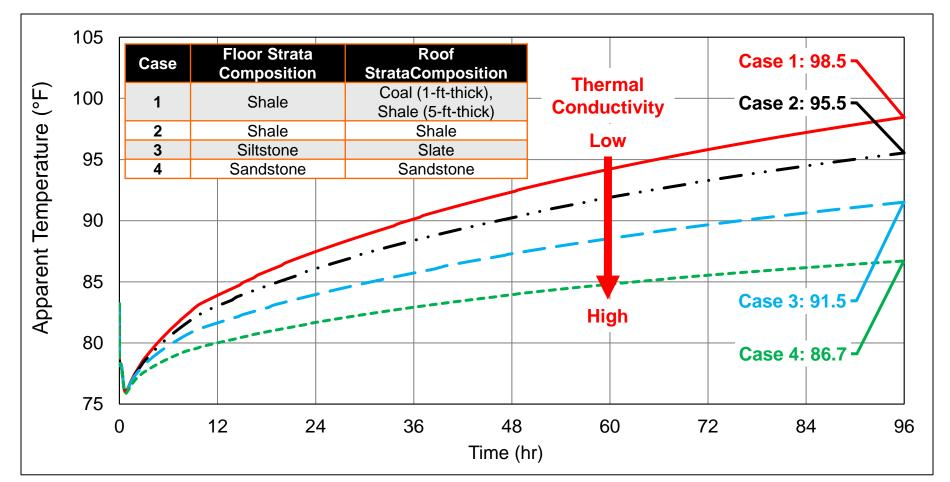
The model was used to evaluate the *mine entry size* (*clearance around RA*) on the predicted RA air temperature after 96 hours
