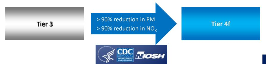
MSHA engine certification data [MSHA 2018b] indicate that replacing older engines with adequate engines certified after January 2015 could result in lower ventilation rate requirements.
