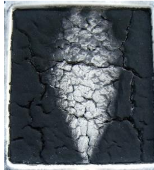
Coal dust on top of untreated rock dust (Exposed to water and dried)
