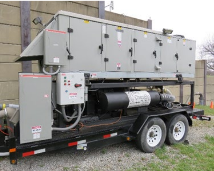
Borehole Air Supply w/ Air Conditioning
