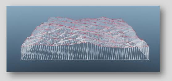
The likelihood of collision/interactions will be estimated through probability fields. The basic idea is that trajectory profiles are projected through time using a Normal distribution or a composite created through kernel density estimation. The overlap in profile determines the likelihood of interaction between two objects.
