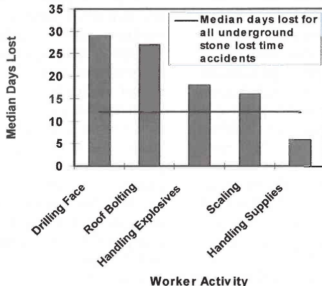
Figure 9 - Median days lost for lost-time groundfall incidents in underground stone mines base on worker activity (MSHA, 1983-1999)
