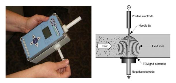
A sampling device used by industrial hygienists to characterize hazardous airborne particulate matter to investigate
