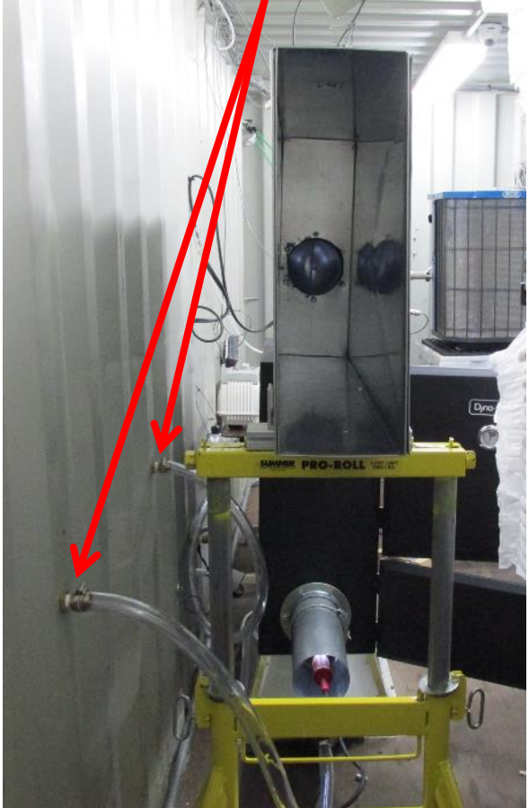
Air Line Bulkhead Fittings
