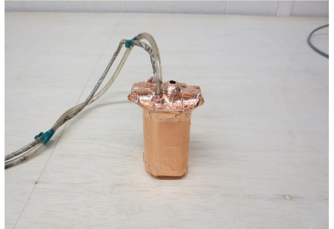
Copper foil (0.00064") shielding
