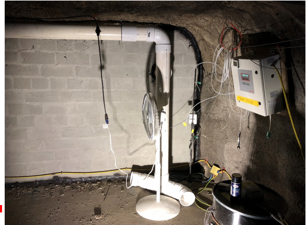
L-shaped air inlet for VSC #6
