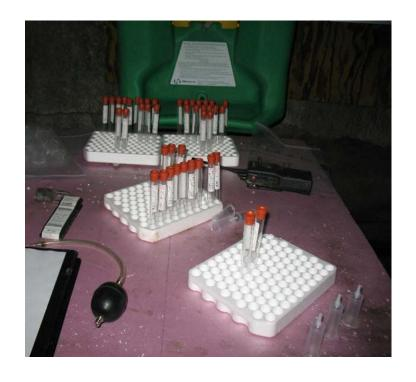
Test results: 2-3% of  $SF_6$  entered RA after 5-30 test subjects entered RA from  $SF_6$  atmosphere with/without blower active (10,000 ppm CO atmosphere would equate to 200-300 ppm entering RA)
