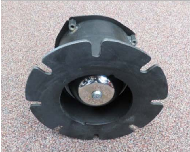
4-inch blast valve
