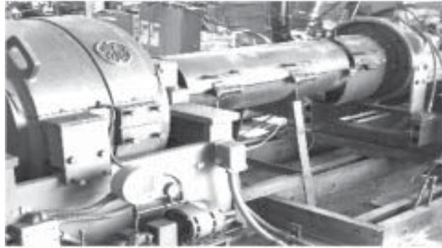
Figure 6: Diesel Engine Shaft Guard Between Dynamometer and Engine
