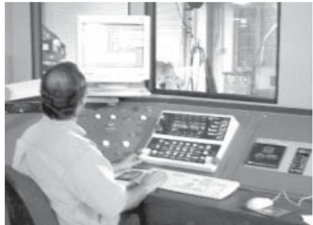
Figure 2: New Super Flow Dynamometer Control & Data Acquisition System
